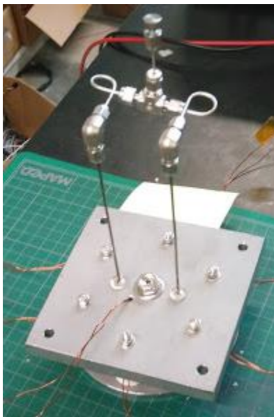
Figure 19 - This image shows the back of the thruster with the final components of the gas delivery system. This includes one T fitting and two 90° elbow fittings. About 4 in of tubing are left exposed in the event the Swagelok fittings need to be destructively removed for disassembly.
