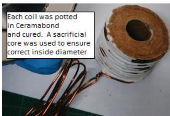
Figure 15 - This shows the center coil. Each coil was potted in alumina Ceramabond™ and cured. The potting allowed for coil modularity during assembly/disassembly.
