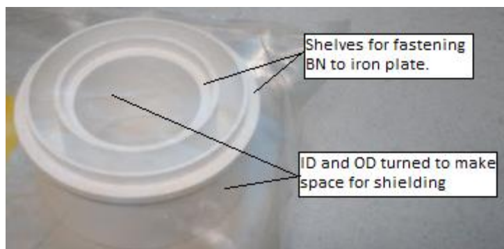
Figure 16 - The BN channel. The channel protects the iron and coils in addition to acting as an electrical insulator.
